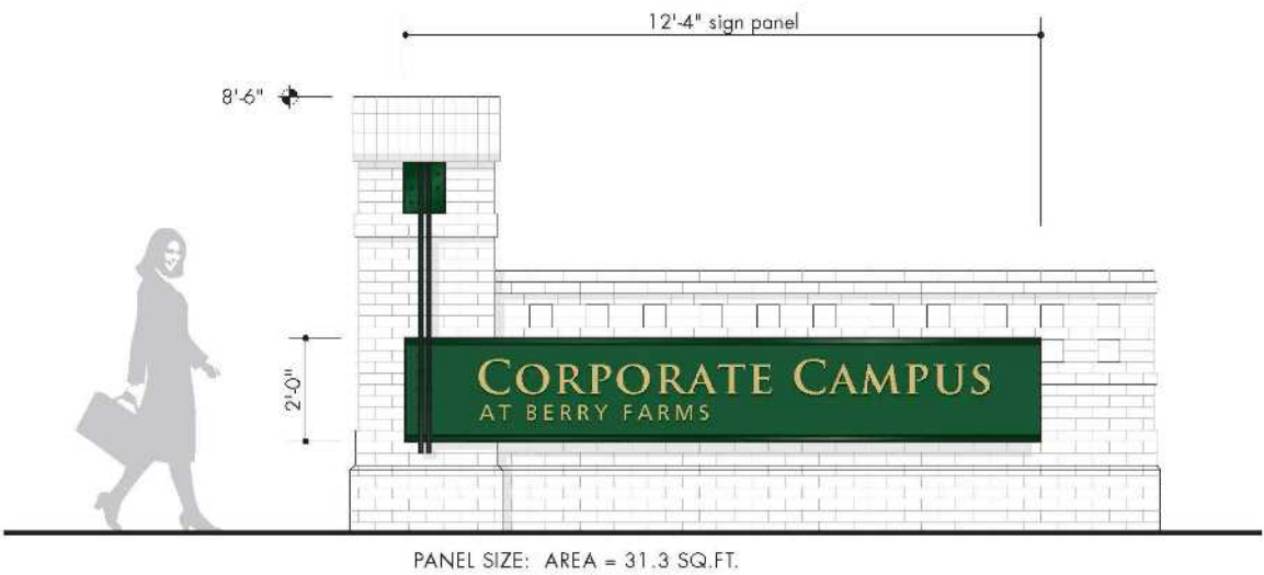
3 2.12 SIGN TYPE 4C: CORPORATE DISTRICT ID . ELEVATION SCALE: 1/4" = 1'-0"
