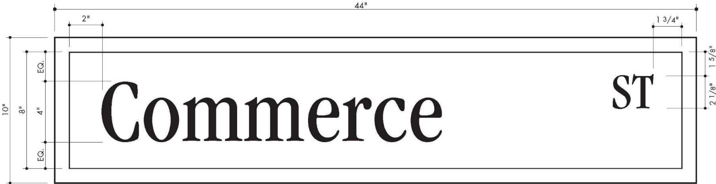
1 2.28 SIGN TYPE 10C - STREET SIGN . DETAIL ELEVATION SCALE: 3" = 1'-0"
