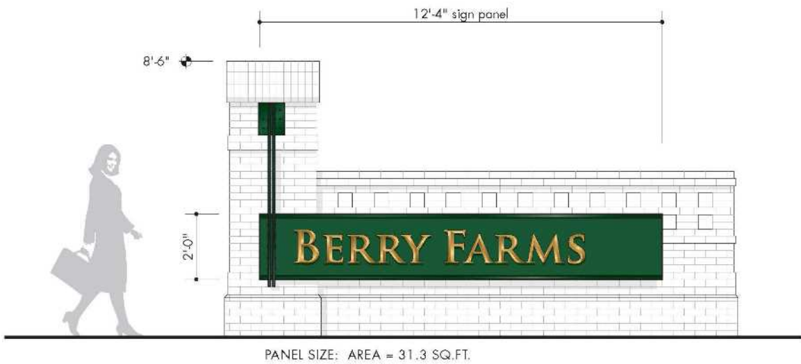
4 2.12 SIGN TYPE 4C: CORPORATE DISTRICT ID . ALTERNATE COPY CONDITION SCALE: 1/4" = 1'-0"
