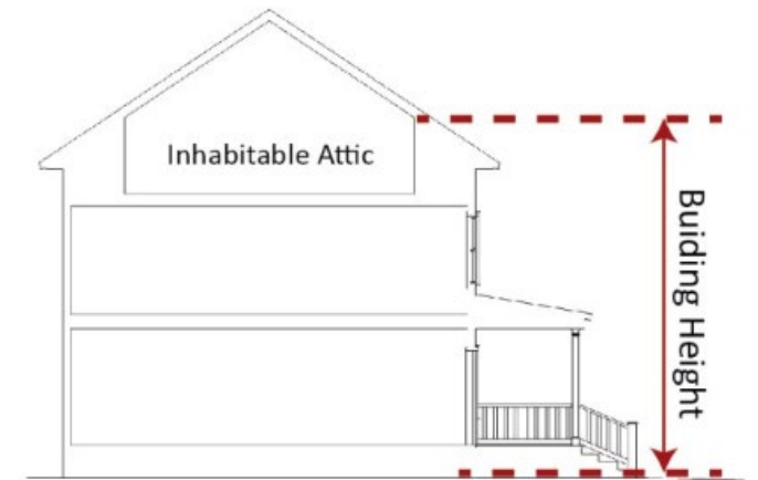
Figure 23.2.3.B Building height with inhabitable attic
