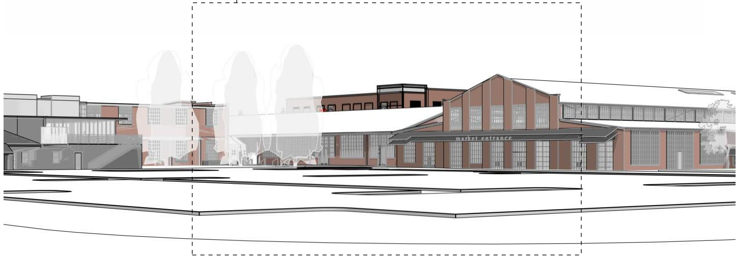
PROPOSED DESIGN PARAPET AT GARAGE TO CONCEAL CARS AT THE TOP LEVEL AS WAS PREVIOUSLY APPROVED
