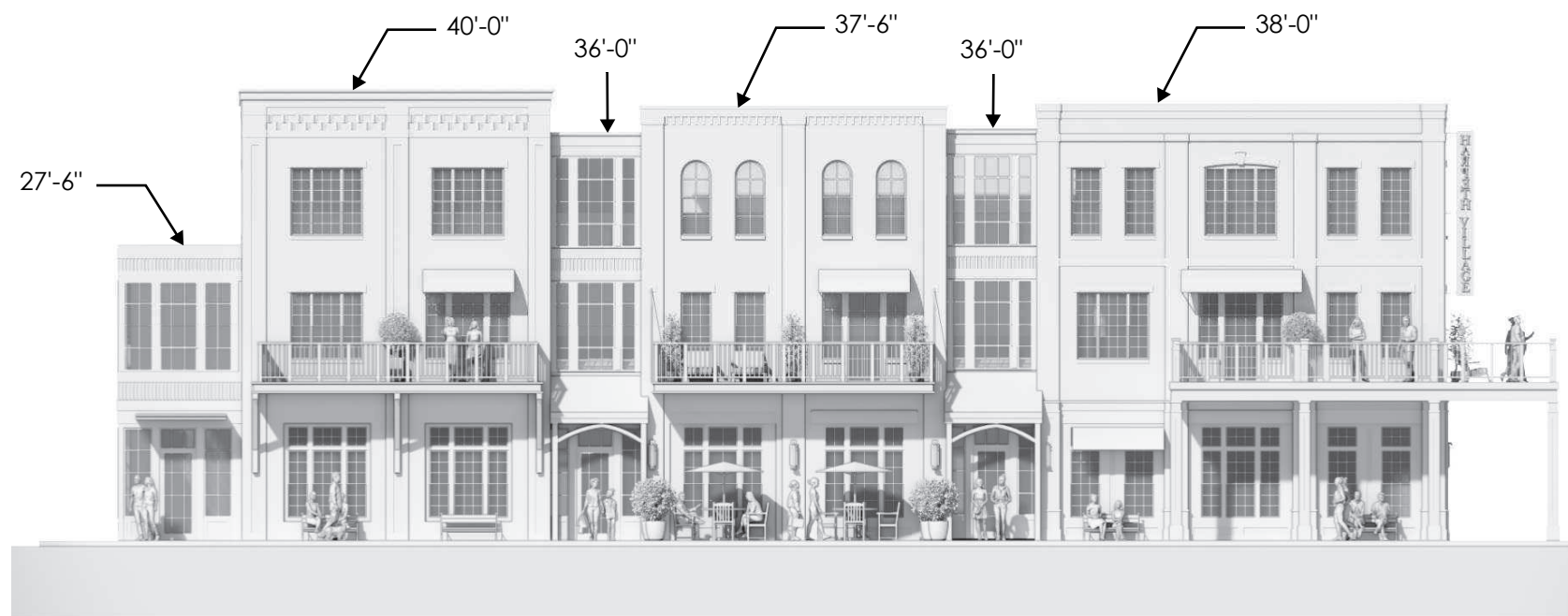
Bldg. - 2 - Elevation-3: Scale 1/16" = 1'-0"
