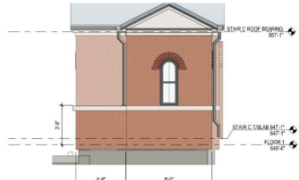
5 EAST ELEVATION - STAIR ENCLOSURE 1/4" = 1'-0"
