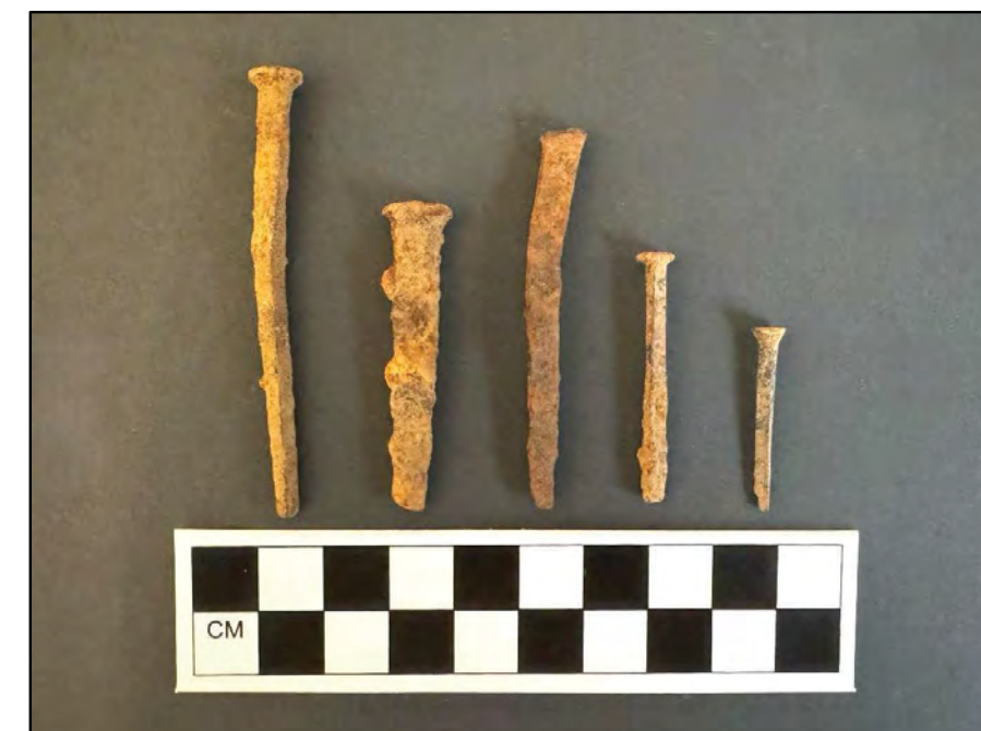
Figure 23. Photograph of selected Type B square cut nails recovered from the site.
