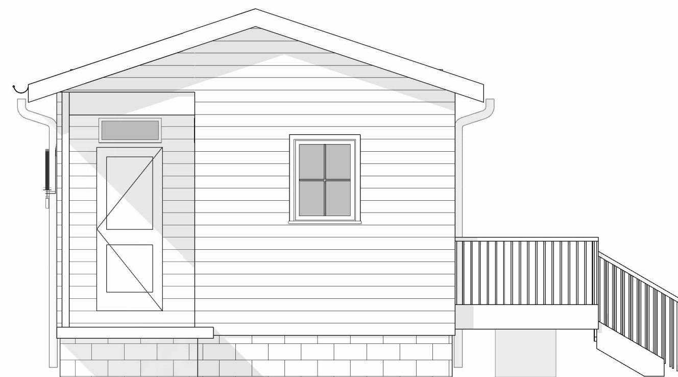
1c EXIST. EXT. ELEVATION - SOUTH 1/4" = 1'-0"
