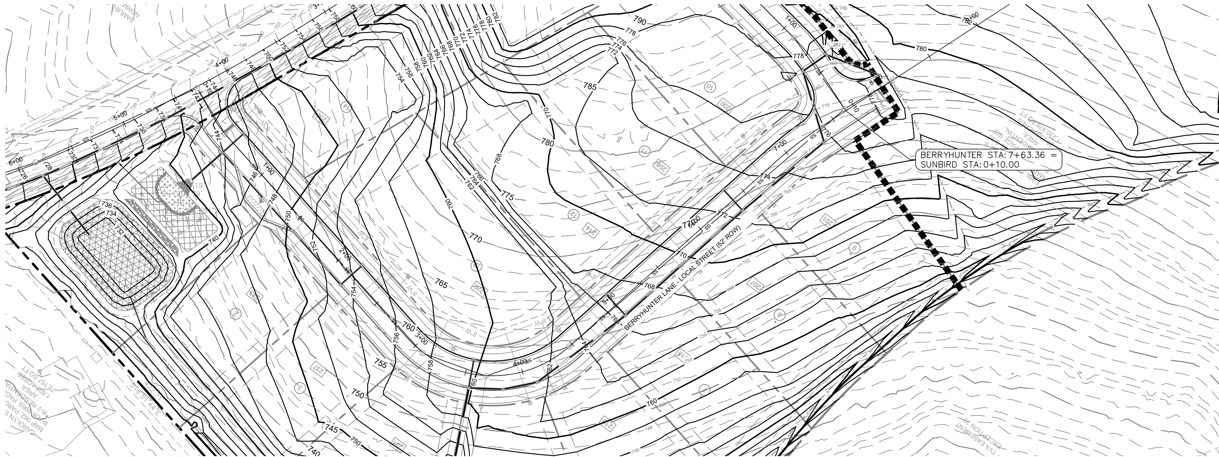
BERRYHUNTER LANE - PLAN VIEW 52' PUBLIC R.O.W. POSTED SPEED = 5MPH, DESIGN SPEED = 30 MPH
