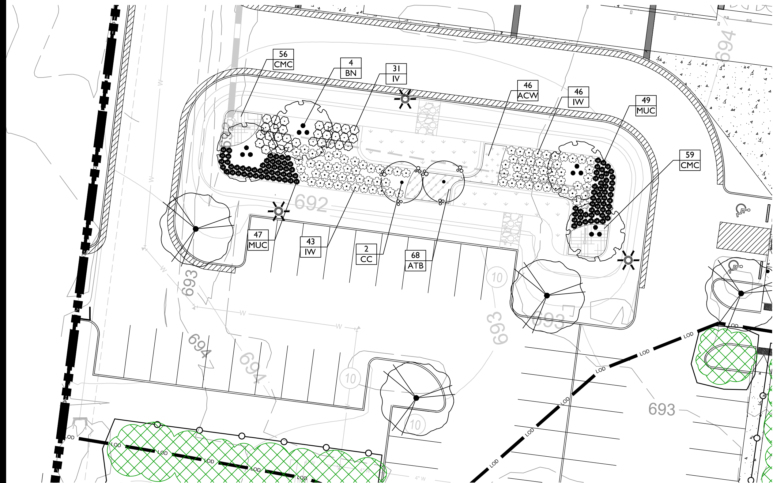
3 L2.3 BIORETENTION AREA 3 - 2,374 SF (LEVEL 1 ORNAMENTAL)
