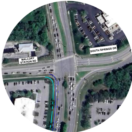
CSG # 6 MALLERY LANE AT MALLERY STATION ROAD/SOUTH SPRINGS DRIVE Adjust the signal timings for the eastbound and westbound approaches to accommodate higher turning movements due to background traffic on Mallery Station Road and due to CoolSprings Galleria site traffic on South Springs Drive.
