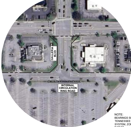
CSG # 16 GALLERIA BOULEVARD AT INTERNAL CIRCULATION RING ROAD The existing ring road west of Galleria Boulevard may be impacted by future greenway and/or sidewalk improvements. The CoolSprings Galleria PUD Subdivision development plan should show any adjustments to lane assignments, pavement markings, multimodal facilities, and roadway/intersection geometry that are needed to accommodate the future greenway and/or sidewalk improvements.
