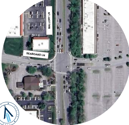
CSG # 9 MALLERY LANE AT SEABOARD LANE Adjust the signal timings for the eastbound and westbound approaches to accommodate higher turning movements due to background traffic growth and CoolSprings Galleria site traffic.
