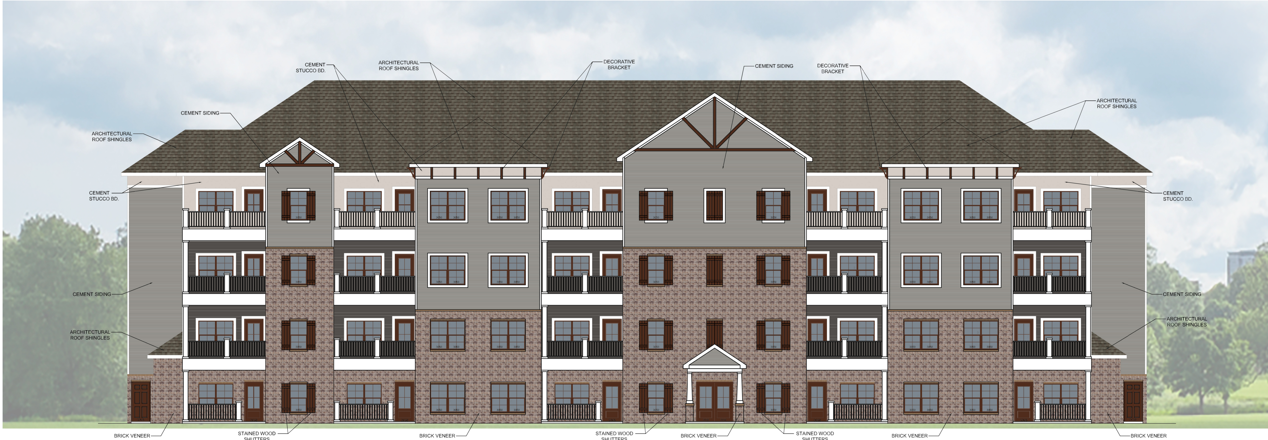
FRONT ELEVATION- Bldg. #4 & #6 Scale: 1/8" = 1'-0"
