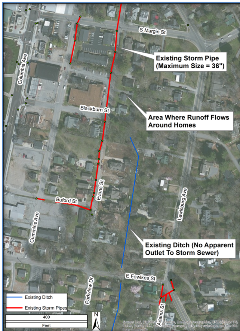
Figure 2: Parkview Site Visit Observations
