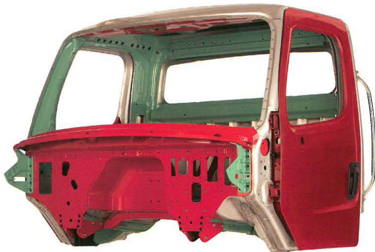
Aluminum Structural Reinforcements E-coated Steel Reinforcements Corrosion-resistant Aluminum Panels
