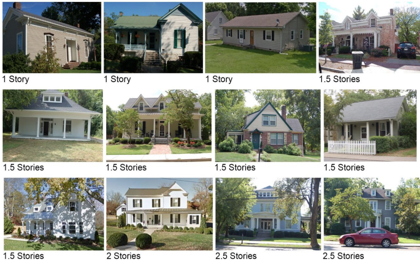
Figure 5-5: These examples depict whole and half-stories for the purposes of determining average height.
