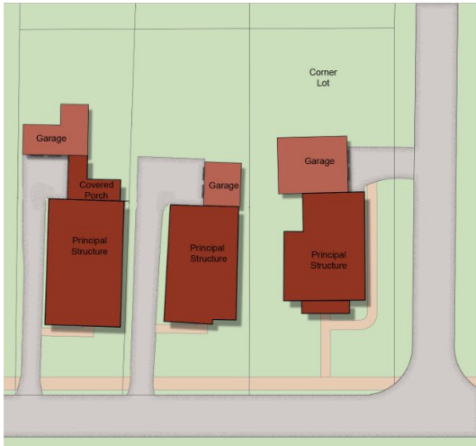
Figure 5-6: These examples show how attached garages are traditionally placed and subordinate to the rest of the principal structure.
