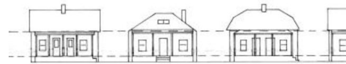
This line of houses demonstrate uniform height.
