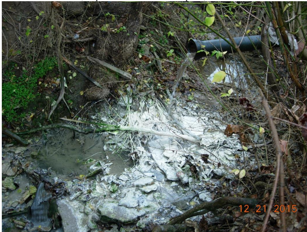
Effluent outfall pipe & discharge, cloudy/opaque effluent discharge, white precipitate & gray deposits in channel leading to receiving stream Fivemile Creek
