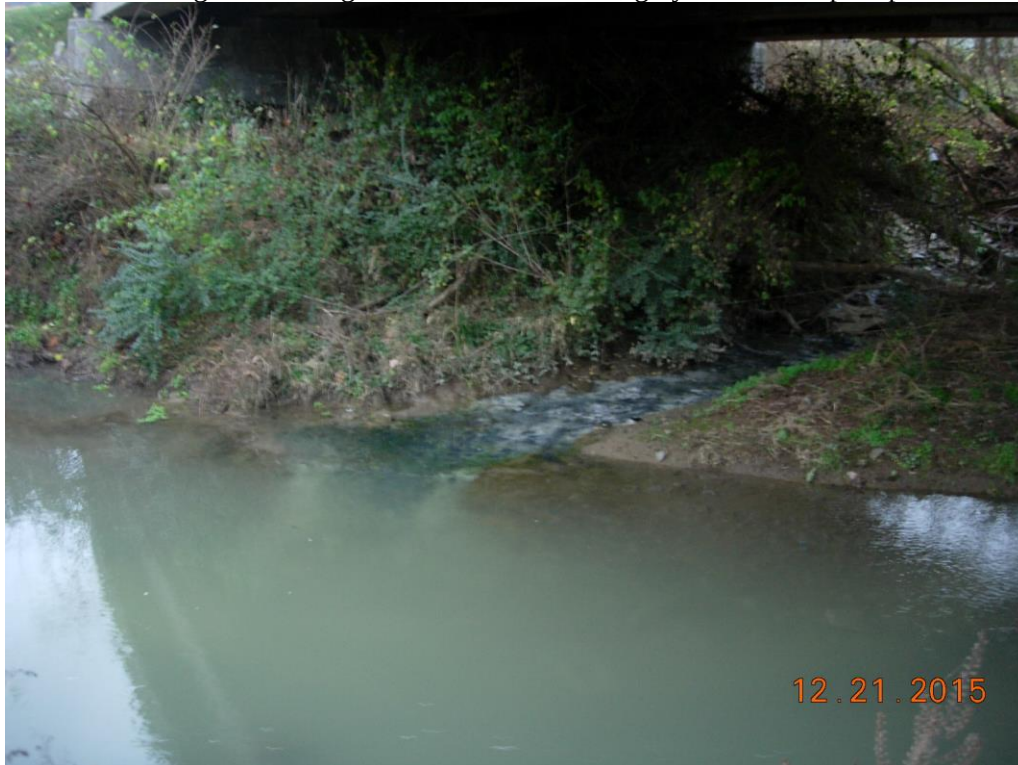
Effluent flow entering Fivemile Creek, showing gray & blackish precipitate & deposits, & discoloration of the receiving stream
