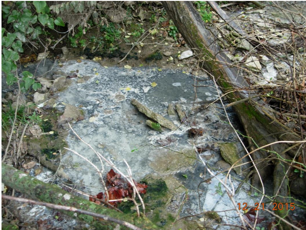
Gray precipitate & deposits in effluent flow
