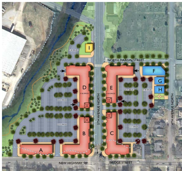
Figure 3-15. Conceptual redevelopment illustrating traditional development standards, mid-block vehicular access, and shared parking.
