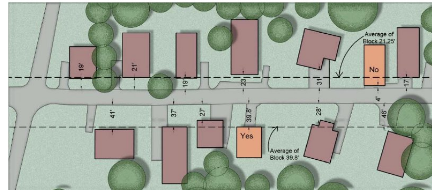
Figure 5-4: The new construction (in tan outlined in red) on the right with a "No" label is not an appropriate average setback for its block face. The dwelling outlined in red on the left with a "Yes" label is an appropriate average setback for its block face.
