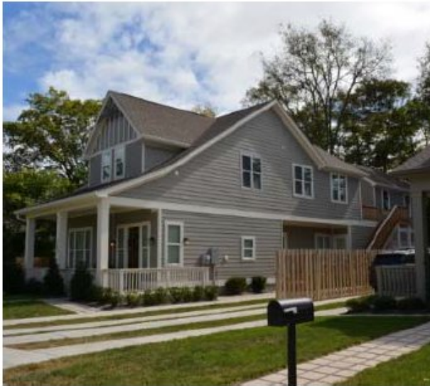
Figure 5-6: These are examples of appropriate design solutions for achieving a one and one-half story appearance at the front elevation.
