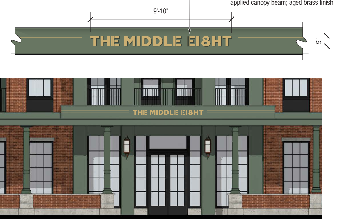
BUILDING 3 WEST ELEVATION DETAIL
