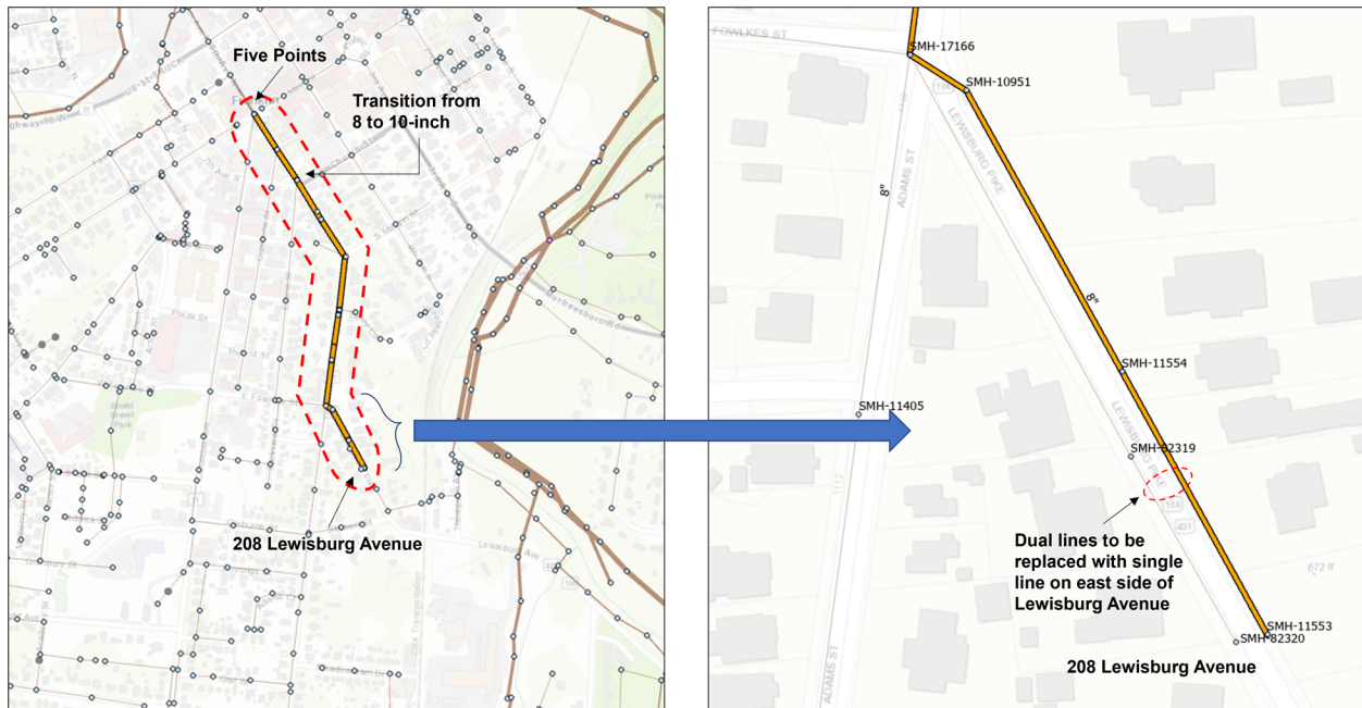
Figure 1: Proposed Sewer Improvements
