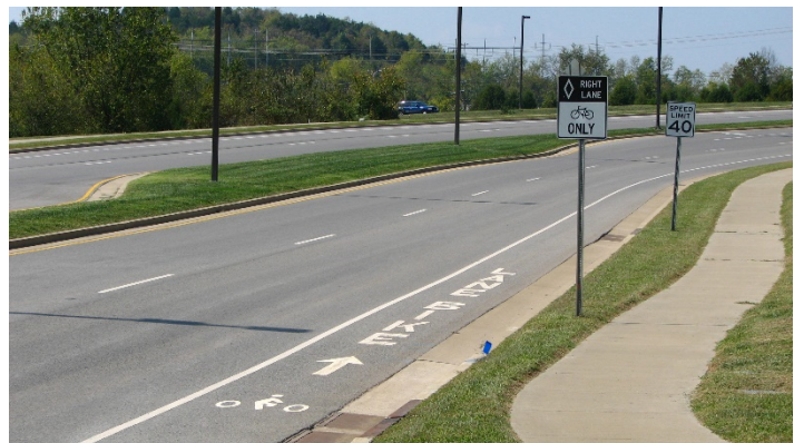
Typical bike lane with signing and markings
