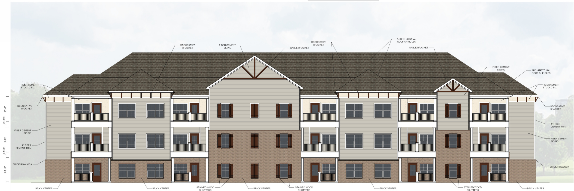
FRONT ELEVATION - Building #7 (30 Units) SCALE: \frac{1}{8}" = 1'-0"
