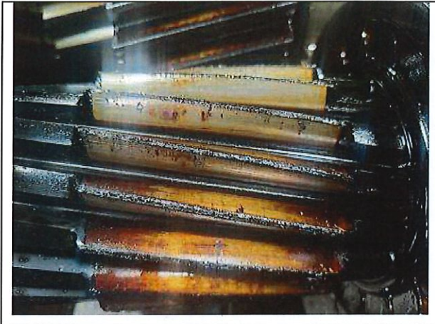
Picture #12: Low speed gear (36.02) is varnished
