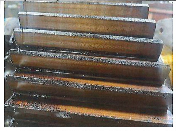
Picture #13: Low speed gear (36.01) is varnished and has corrosion and micro pitting on the gear teeth
