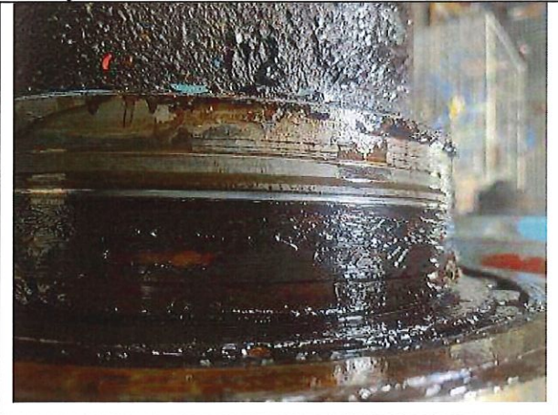
Picture #14: Output collar is grooved at the seal journal
