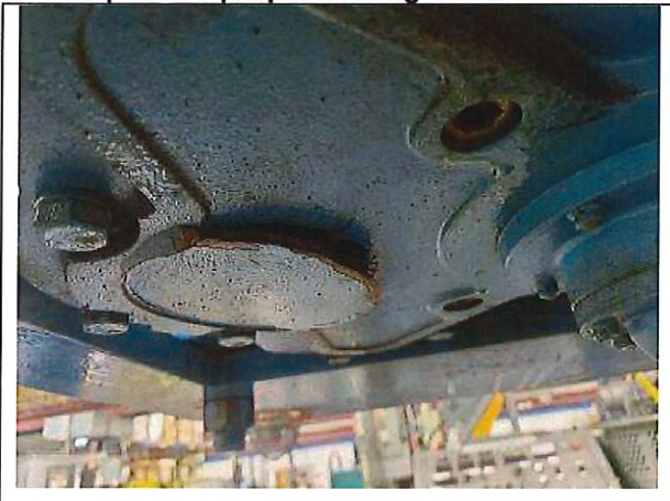
Picture #7: High speed shaft is grooved and corroded
