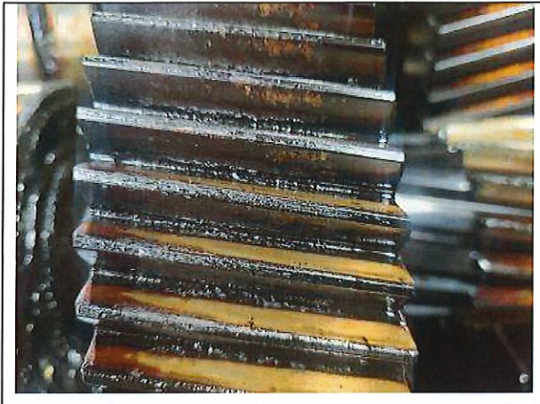
Picture #11: Intermediate gear (36.03) is varnished
