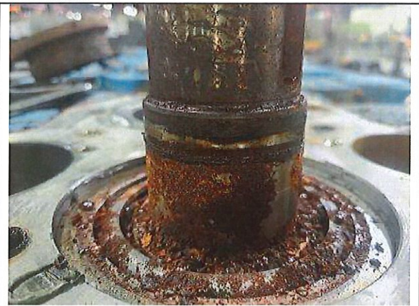
Picture #7: High speed shaft is grooved and corroded
