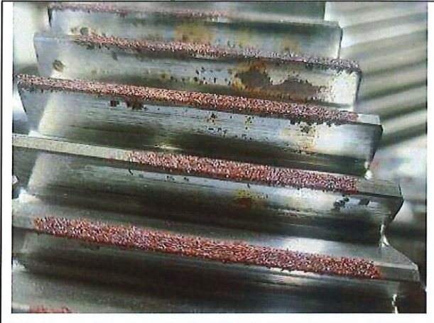
Picture #12: Intermediate gear (36.03) is in good condition
