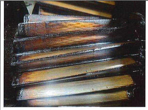
Picture #12: Low speed gear (36.02) is varnished
