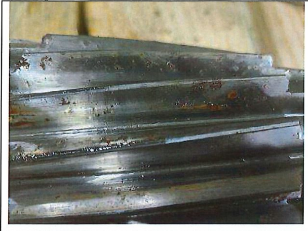
Picture #11: Intermediate pinion (36.04) has surface rust
