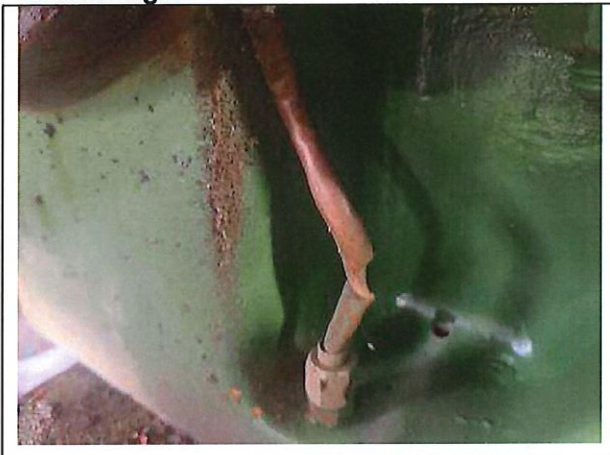
Picture #7: Interior of housing is severely varnished from burnt lubrication
