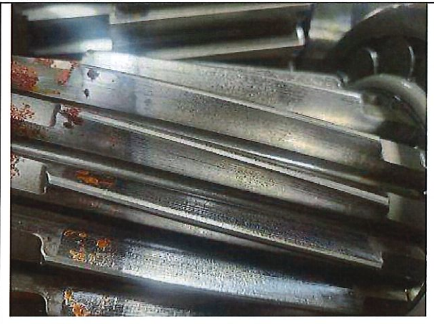
Picture #13: Low speed pinion (36.02) is corroded
