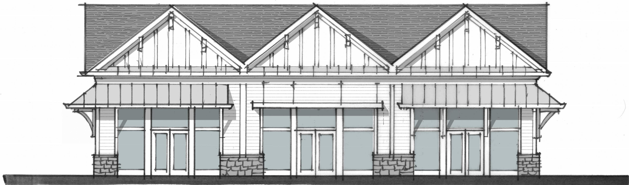
SOUTH ELEVATION View from West Main SCALE: 1/8"=1'
