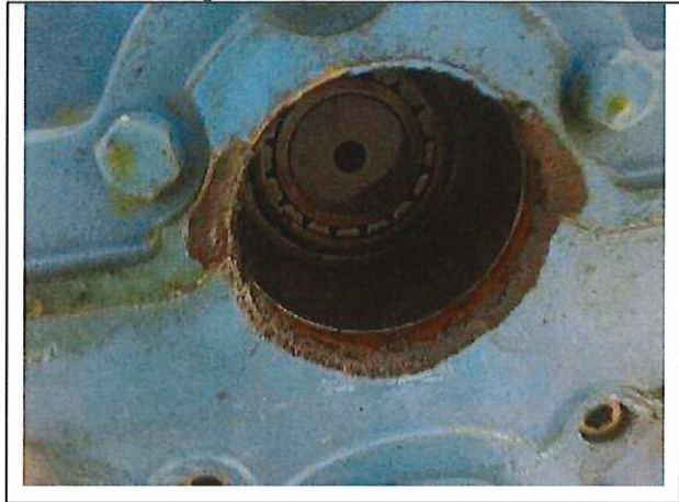
Picture #6: Input gear coupling is corroded
