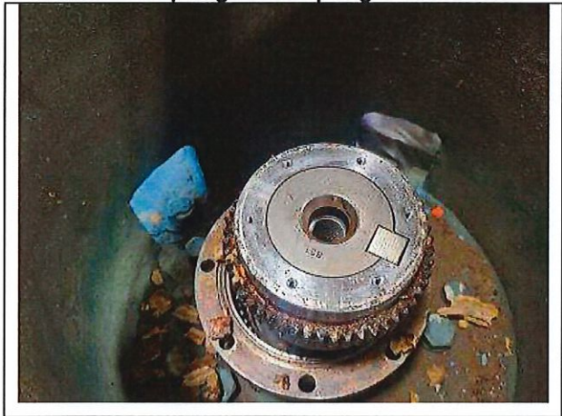
Picture #8: High speed bearings are corroded and will not turn
