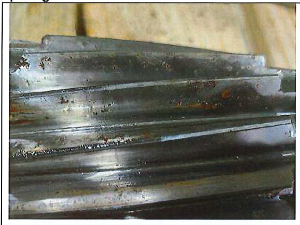
Picture #11: Intermediate pinion (36.04) has surface rust
