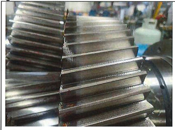
Picture #14: Low speed gear (36.01) has pitting and corrosion
