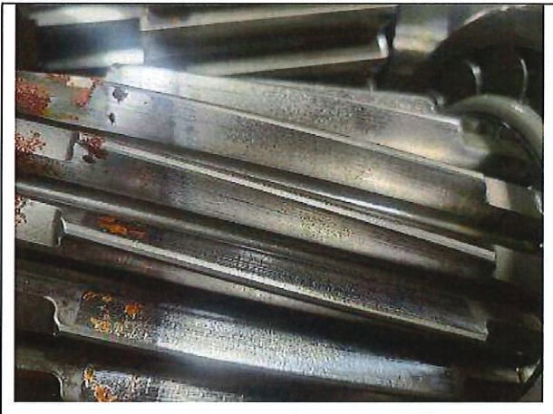
Picture #13: Low speed pinion (36.02) is corroded
