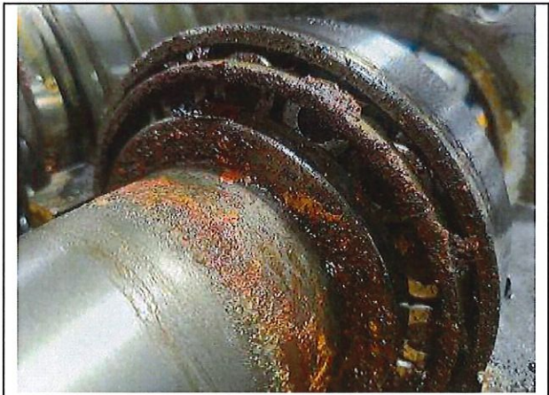
Picture #8: High speed bearings are corroded and will not turn
